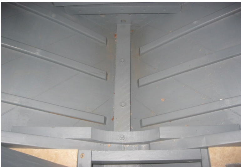
Photo 4 Bottom structure: Keel, webs and stiffeners
