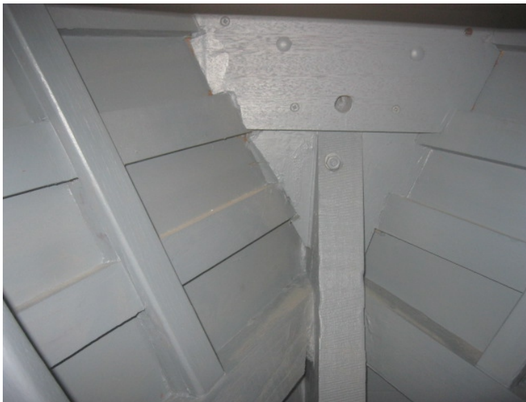
Photo 3 Bow area inside – transfer framing, 2 stringers and 2 longitudinals above WL
