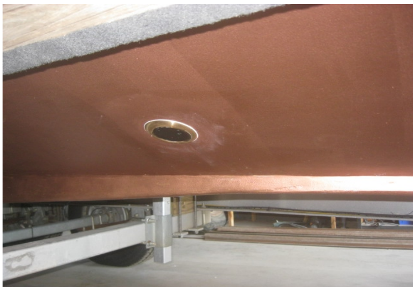
Photo 6 Bottom part appearance with Echo sounder head
